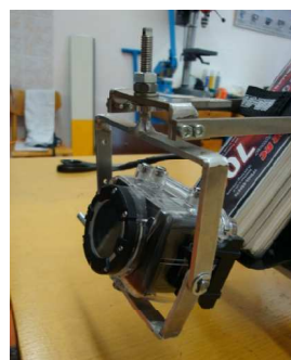
Picture 5 The movable mounting with ActionPro SD21 video camera
